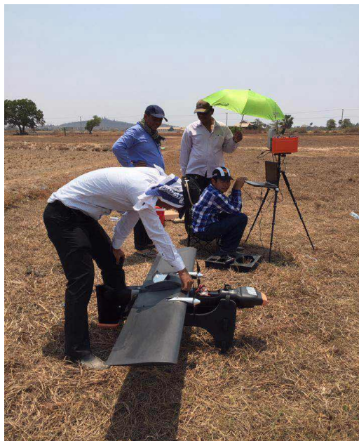
Fig. 32 BDS High-precision Receivers Used for UAV in Cambodia
